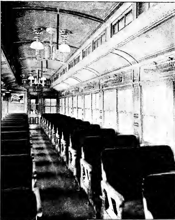
Fig. 94. INTERIOR OF FIRST CLASS COACH. Oil Lamps and Window Blinds.
